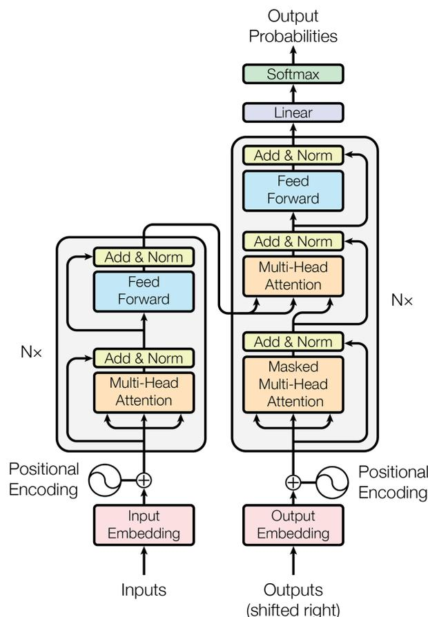
**Figure 2.1:** The original Transformer model architecture by Vaswani et al. (2017).
