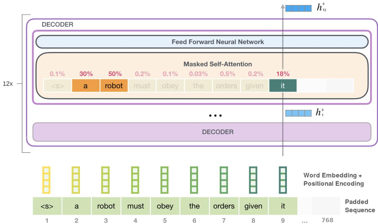
**Figure 2.2:** An overview of the forward pass in GPT-2. Adapted from Alammari (2018b).
