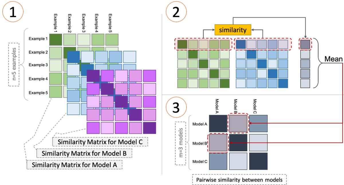
**Figure 2.5:** The Representational Similarity Analysis (RSA) algorithm applied to the representations of three models. Image taken from Abnar (2020).
