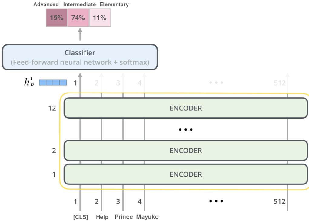
**Figure 2.3:** Using a pretrained ALBERT model for the ARA task. Adapted from Alammari (2018a).
